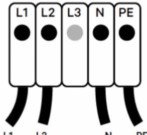
**F.** Ensure that the maximum voltage is less than 264 V between L & N inputs.
